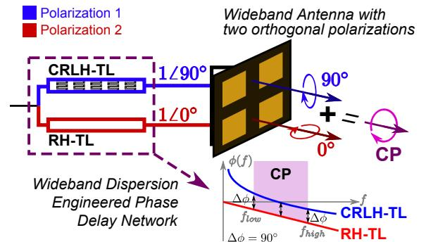
Fig. 1. A general wideband CP antenna system using a CRLH transmission line to provide  $\Delta\phi = 90^\circ$  with respect to a right-handed transmission line (RH-TL). This wideband phase delay network enables CP by feeding a multi-polarized antenna with the proper phase and magnitude.
