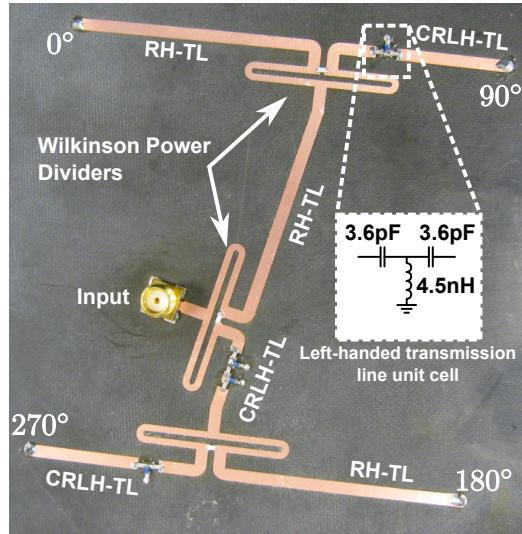
Fig. 2. Prototyped CRLH feed network used to achieve wideband CP radiation. The first power dividing/CRLH stage provides  $180^\circ$  phase delay between the two branches, and each subsequent stage provides  $90^\circ$  phase.
